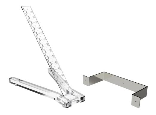
A set of simple tools dedicated for measurements on tomography X-Ray equipment. It can be used for the layer height adjustment and tomography movement tests.
