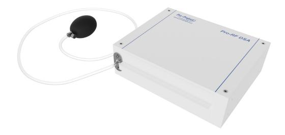
A special phantom for Quality Assurance of Digital Subtraction Angiography Equipment (DSA) according to IEC 61223-3-3 and DIN 6868/Parts 8, (2007) and 54. The phantom contains a movable insert with aluminium strips to simulate blood vessels. This insert can be moved via pneumatic system from a safe distance during exposure.
