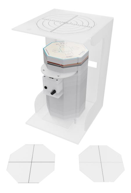
The phantom has been designed in accordance with the NEMA XR21 standard. This modular phantom made of PMMA consists of several plates allowing variation of phantom thickness setup in steps of 25 mm, up to a total of 300 mm, simulating a range of patient sizes.
