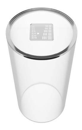
A simple test device for the focal spot size evaluation. It consists of a precision bar pattern placed at the end of the cylinder that provides accurate and reproducible target-to-image receptor spacing.
