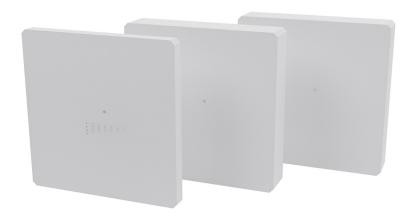
The phantom for acceptance and constancy testing of **Cone-Beam CT / Volume Tomography (DVT) in fluoroscopy** according to **DIN 6868-150**.
