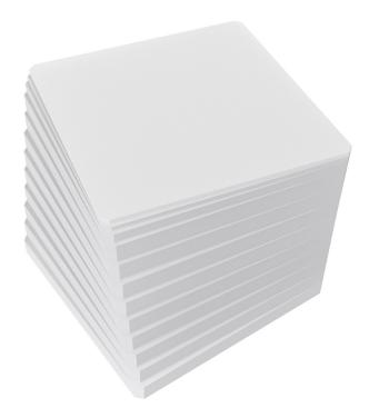
A set of acrylic plates for testing Automated Exposure Control of radiography equipment.
