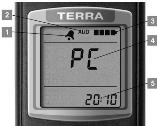
Figure 27 – LCD of the dosimeter (the mode of data communications control with the PC)
