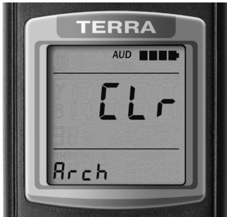
Figure 31 – LCD of the dosimeter (the submode of measurement results clearing stored in the nonvolatile memory)
