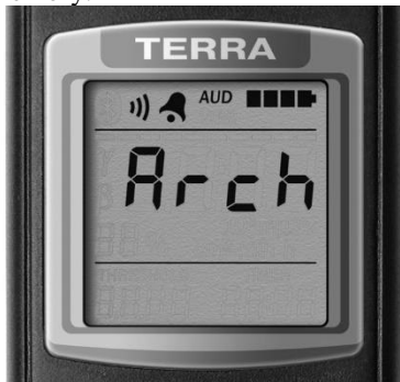
Figure 5 – LCD of the dosimeter (start of the submode of measurement result saving in the nonvolatile memory)
