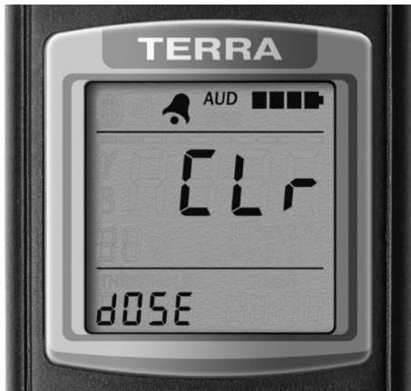
Figure 13 – LCD of the dosimeter (the sumcode of DE and DE accumulation time values resetting)
