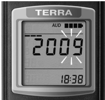
Figure 23 – LCD of the dosimeter (the submode of time and date correction – year programming)
