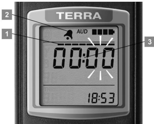
Figure 26 – LCD of the dosimeter (the submode of alarm clock activation time programming)
