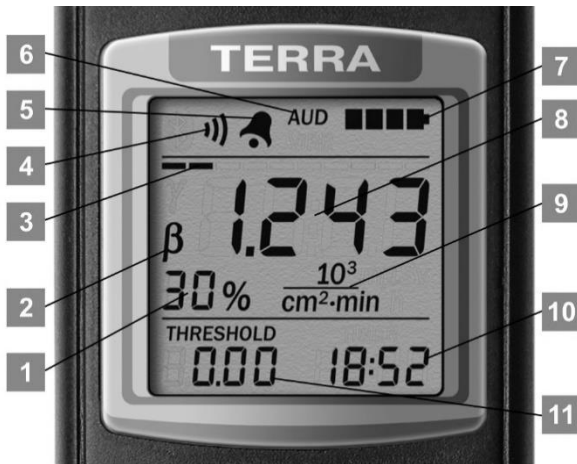
Figure 14 – LCD of the dosimeter (the mode of surface beta-particles flux density measurement)
