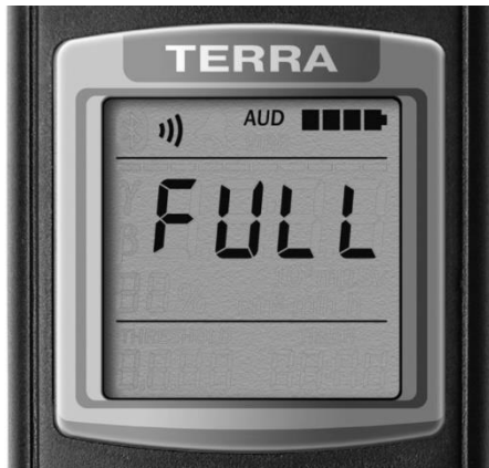
Figure 9 – LCD of the dosimeter (start of the submode of measurement result saving – no free space in the nonvolatile memory)
