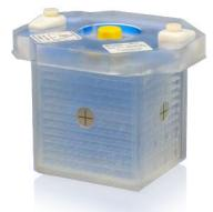
**Above:** The QUASAR GRID<sup>3D</sup> acrylic cube containing a 1cm 3D grid of 1.5 mm channels filled with CuSO, solution.
